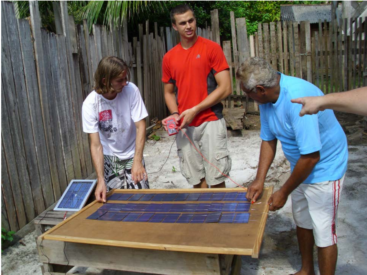
Mike testing the set of 36 finished PV cells that will make a 65 watt module. A finished solar cell phone charger is setting over to the left, recharging somebody's cell phone.
