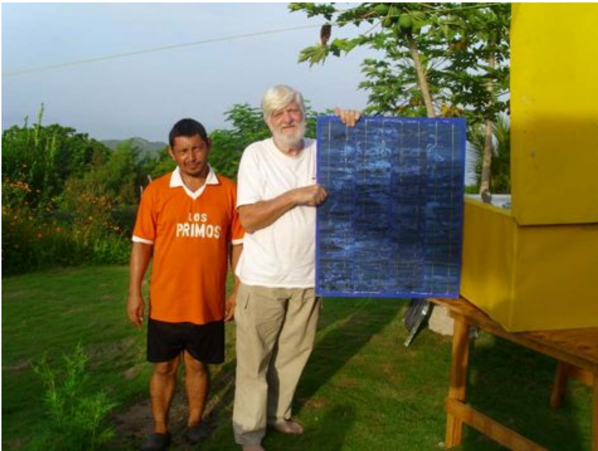
Hugo and I with the successfully encapsulated 65 watt PV module right out of the oven. You can see the grain of the polycrystalline silicon Evergreen solar cells. The module works perfectly.
