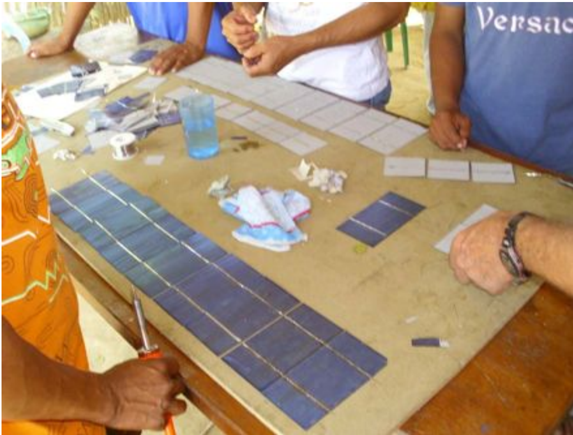
Soldering strings of whole PV cells to make a 65 watt PV module
