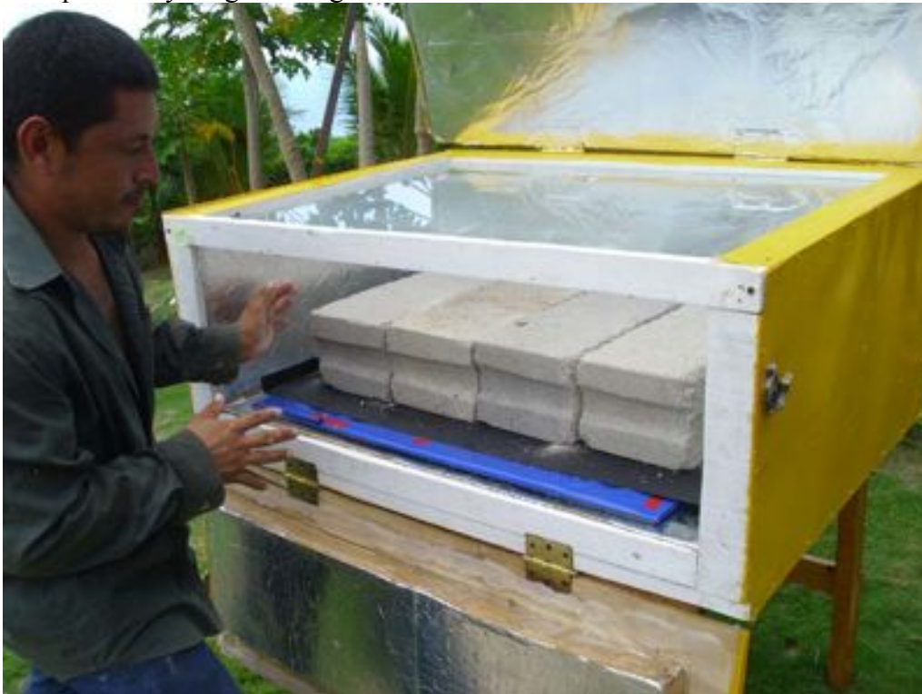
The EVA PV module sandwich in the solar cooker ready for baking at 120° C
