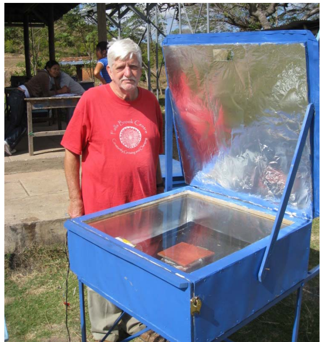
Fig 1 Richard Komp with the solar oven used for laminating the PV modules, showing the clay tile platen used under the module sandwich. This platen has electric heating elements buried in the middle.
