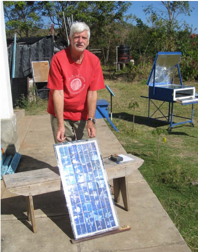
Fig 4. Rich Komp Testing the 32 Watt PV module made in the larger solar laminating oven with the small laminating oven in the background.
