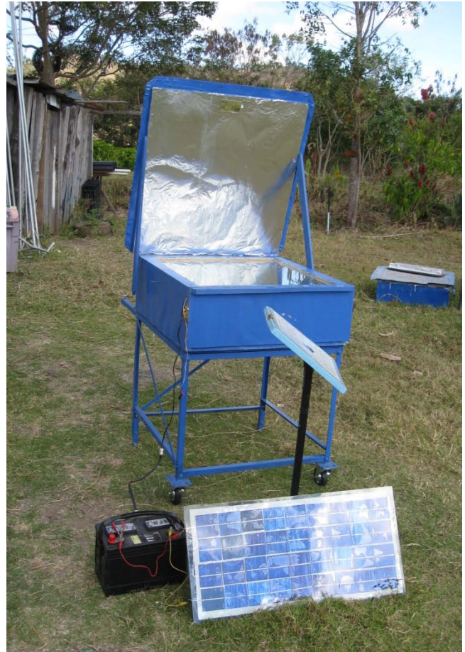
Fig 5 The 32 Watt EVA encapsulated PV module charging a 12 volt storage battery being used to power the experimental solar electric platen heating the solar oven used to laminate the PV modules. The module still needs its aluminum frame.
