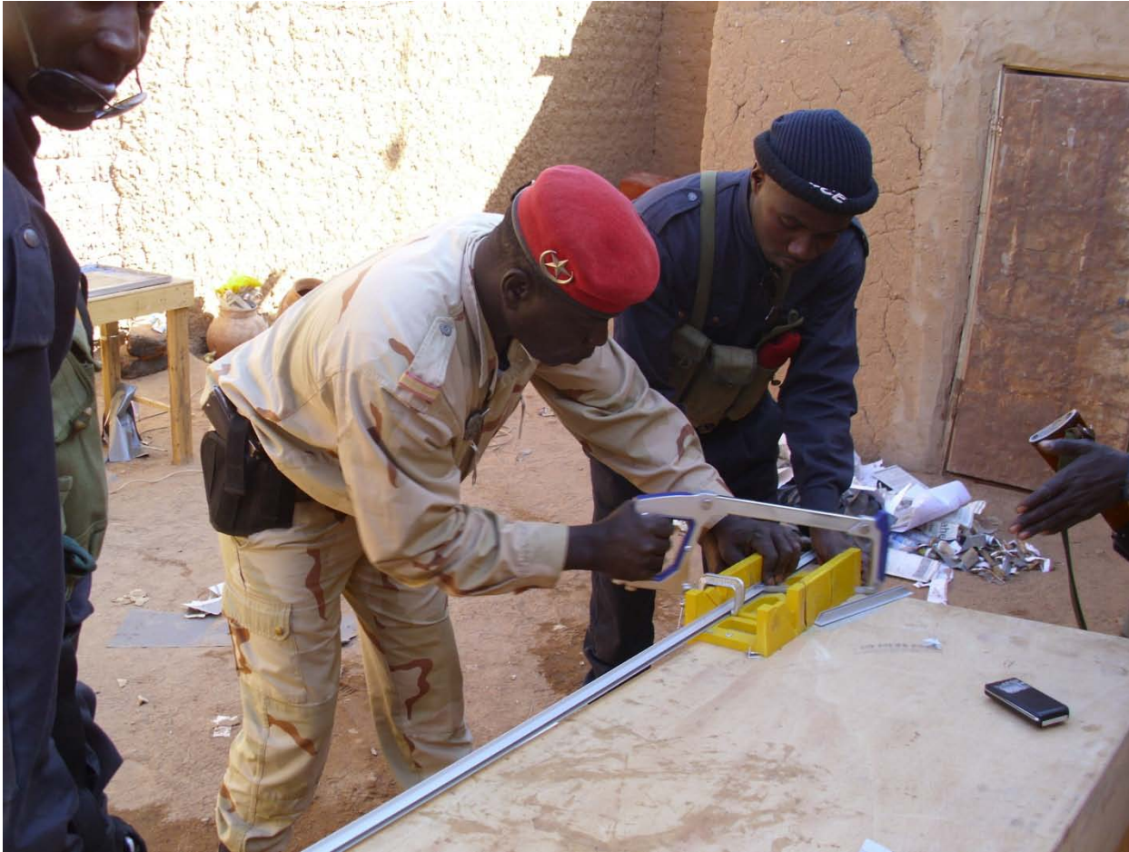
Some of the soldiers taking part in the workshop, cutting frames for the cell phone chargers.
