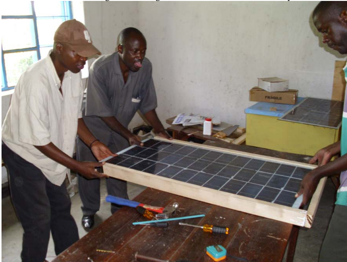
Sliding a finished 60 watt PV module into one of the frames made by the orphans. The new wooden frame design developed by one of the genocide survivors (who is an excellent carpenter) is stronger but easier to make than the design we were using.
